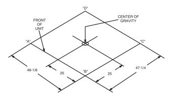
FIGURE 2 - UNIT CENTER OF GRAVITY
